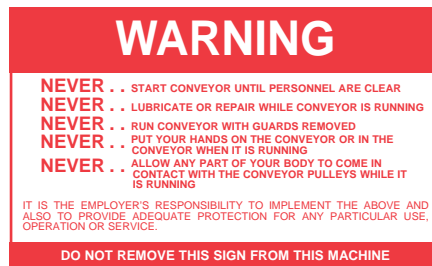
PLACED AT DRIVE OF ALL POWERED CONVEYORS.
